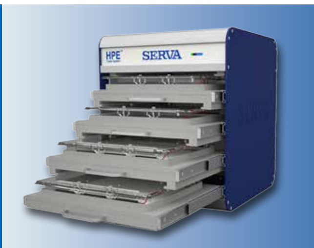
The HPE™ BlueTower is a multilevel flatbed electrophoresis device providing unmatched resolution and reproducibility in horizontal IEF.
